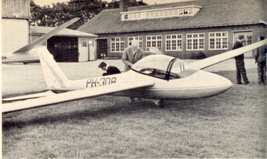
Single-place, privately owned, Dutch-designed Sagitta sailplane is assembled at the Terlet Gliding Center. Some 145 sailplanes are registered in Holland, majority of which are German Schleicher K-6, K-7, and K-8 series
