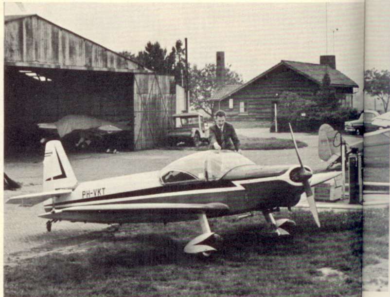
W. B. Burgstede, assistant manager and chief instructor at Teuge field, closes canopy of privately owned Scintex Emeraude CP-317, a French-designed plane powered by a 90-h.p. Continental engine. Piper J-3 in background is used for instruction by the Dutch National Flying School (NLS)
